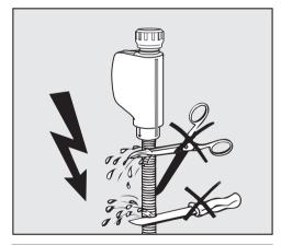
⚠ Do not cut the inlet hose or damaged it in any way.
